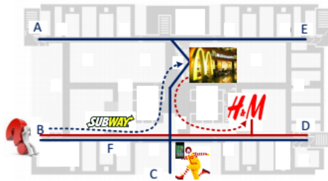
Figure 2.2: A usage scenario of Travi-Navi. McD collects traces along aisles in blue, and those by HM are in red. A shortcut (with a red dashed line) between McD and HM is identified from two guiders' traces. [2]
