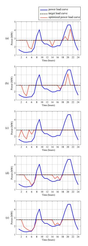
**Figure 8.** Optimized power load curves with 60% *TLC*<sub>*pct*</sub> and *SOC*<sub>*i*,*ave*</sub> of (**a**) 40%, (**b**) 50%, (**c**) 60%, (**d**) 70% and (**e**) 80%.
