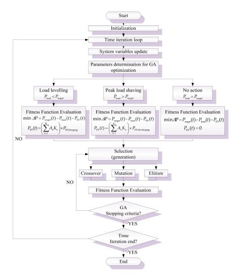
Figure 5. Flowchart for the proposed V2G optimization algorithm.
