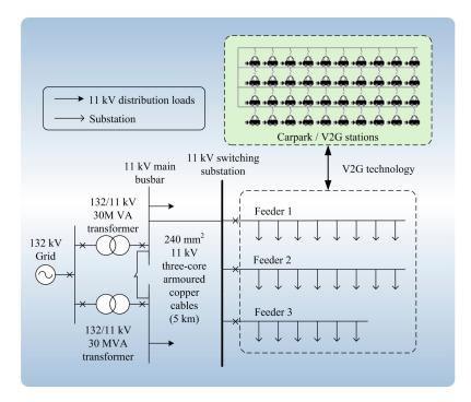
Figure 2. Single-line diagram of a generic township.
