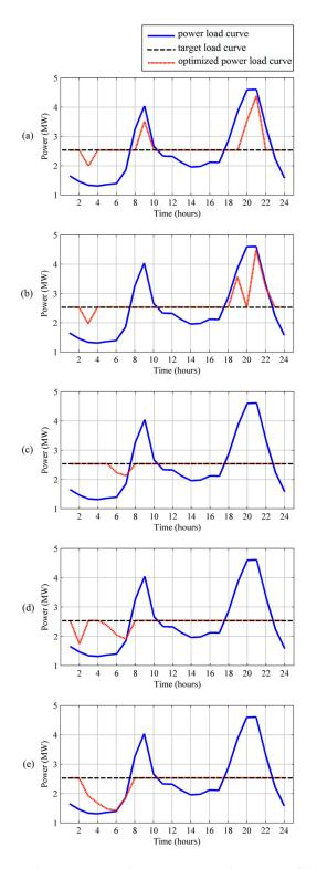
**Figure 7.** Optimized power load curves with 55% *TLC*<sub>*pct*</sub> and *SOC*<sub>*i*,*ave*</sub> of (**a**) 40%, (**b**) 50%, (**c**) 60%, (**d**) 70% and (**e**) 80%.
