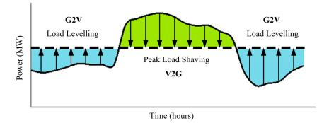
Figure 3. The concept of peak load shaving and load levelling.
