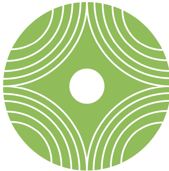
Figure 37. SynRM with axially laminated rotor [23].
