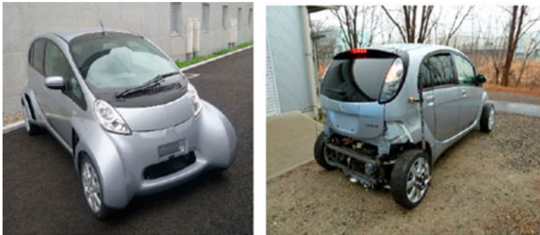
Figure 15. Experimental vehicle with W-IWM system by Sato et al. [26]. (Reprint with permission [26]; 2015, IEEE.)
