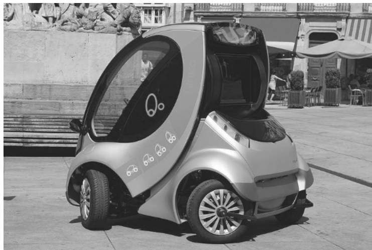
Figure 14. Hiriko Fold—a vehicle employing in-wheel motors.
