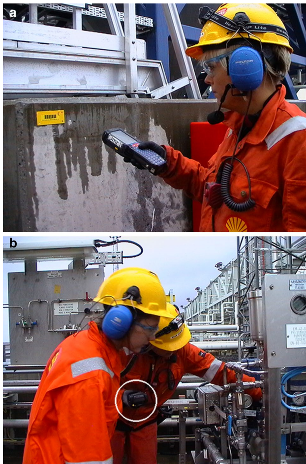
Fig. 4 Ergonomic challenges related to scanning with a PDA: a aligning the scan exit window correctly and detecting the laser beam; b the device's constant presence
