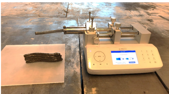
Fig. 3. A high-pressure syringe pump is utilized for 3D-printing the samples.
