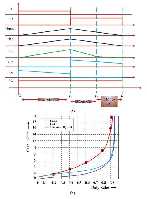
**Figure 3.** (a) Mode diagram of the proposed circuit; (b) voltage gain versus duty ratio for boost, Cuk and proposed hybrid converter.
