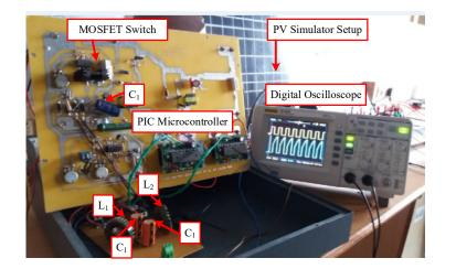
Figure 19. Prototype setup of the proposed converter.
