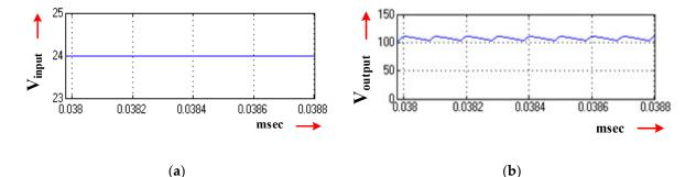
**Figure 14.** Simulation waveforms for input voltage 24V DC and 0.8 duty cycle; (**a**) input voltage waveform (voltage scale: 1 V/div and t: 20  $\mu$ s/div) and (**b**) input voltage waveform (voltage scale 50 V/div and t: 20  $\mu$ s/div).
