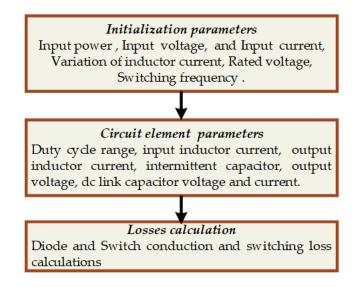
Figure 13. Design setup of converter parameter selections.
