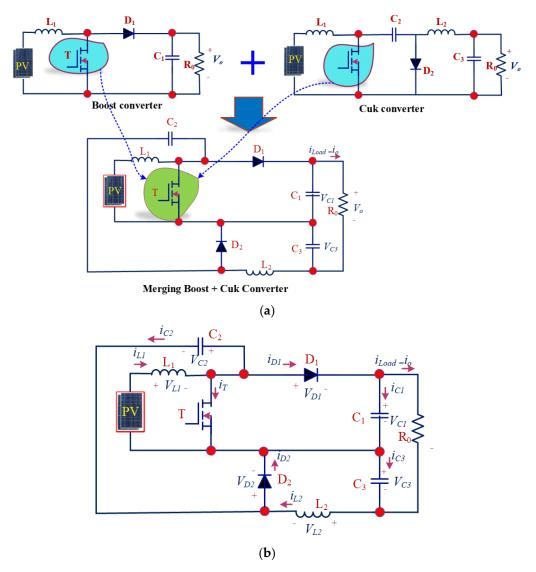
Figure 1. (a) Proposed converter integration; (b) proposed single switch hybrid DC–DC converter.
