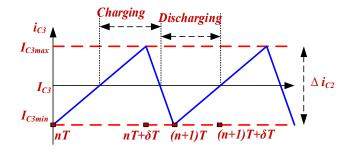
Figure 6. Capacitor current ic3.
