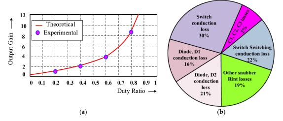
**Figure 26.** (a) Theoretical and experimental results comparison. (b) Experimental power loss distribution operating at rated condition (duty ratio from 0.8).
