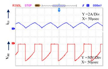
**Figure 25.** The experimental waveform of the input inductor current, *i*<sub>L1</sub> and voltage across *i*<sub>D2</sub> the power switch for input voltage 24 V and 0.8 duty cycle.
