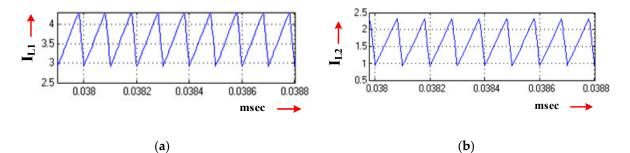
**Figure 16.** Simulation waveforms for input voltage 24 V DC and 0.8 duty cycle; (**a**) inductor current  $i_{L1}$  waveform (current scale: 0.5 A/div and t: 20 µs/div) and (**b**) inductor current  $i_{L2}$  waveform (current scale: 0.5 A V/div and t: 20 µs/div).
