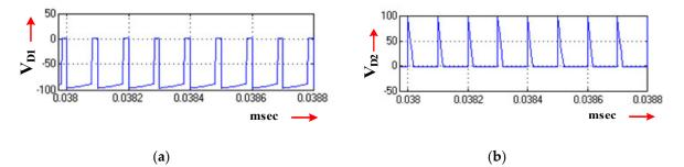
**Figure 17.** Simulation waveforms for input voltage 24V DC and 0.8 duty cycle; (**a**) voltage across the power diode, V<sub>D1</sub> waveform (voltage scale: 50 V/div and t: 20  $\mu$ s/div) and (**b**) voltage across the power diode, V<sub>D2</sub> waveform (voltage scale: 50 V/div and t: 20  $\mu$ s/div).
