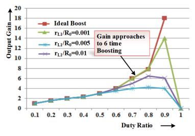
Figure 12. Voltage output gain versus duty cycle.
