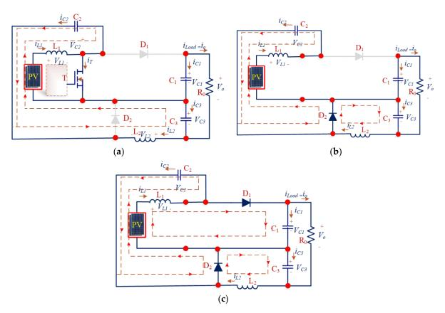
**Figure 2.** Modes of operation of the proposed hybrid DC-to-DC converter: (**a**) Mode- I [t<sub>a</sub>-t<sub>b</sub>]; (**b**) Mode- II [t<sub>b</sub>-t<sub>c</sub>]; (**c**) Mode- III [t<sub>c</sub>-t<sub>d</sub>].
