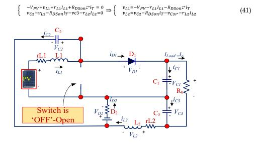
Figure 11. Equivalent circuit of the converter with losses in mode-2 and mode-3 operation.
