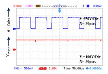
Figure 20. The experimental waveform of the duty cycle and input voltage.
