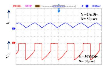
**Figure 24.** The experimental waveform of the input inductor current, *i*<sub>L1</sub> and voltage across *i*<sub>D1</sub> the power switch for input voltage 24 V and 0.8 duty cycle.
