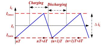
Figure 8. Evolution of the inductor current.
