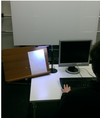
Figure 3: A photo of the experiment setup including a user, the book rest, screen, and keyboard for performing the transcribing task and the projection canvas behind which the loudspeakers were placed. When display Location was dorsal, the position of the chair, desk, and book rest were rotated 180° so that the distance to the projection screen and loudspeaker did not change but these were now at the participants' back. Texts used when transcribing contained random word sequences of the same difficulty out of a pool of 72154 lowercase words without accents or special characters. A different text was used in each dual-task condition, which remained the same for all participants in each experiment session.
