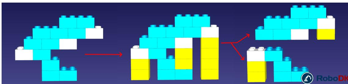
Figure 3.12: Another example from Sugimote et al.'s thesis recreated in RoboDK, this example combines both support blocks and sub-figures to build a difficult shape
