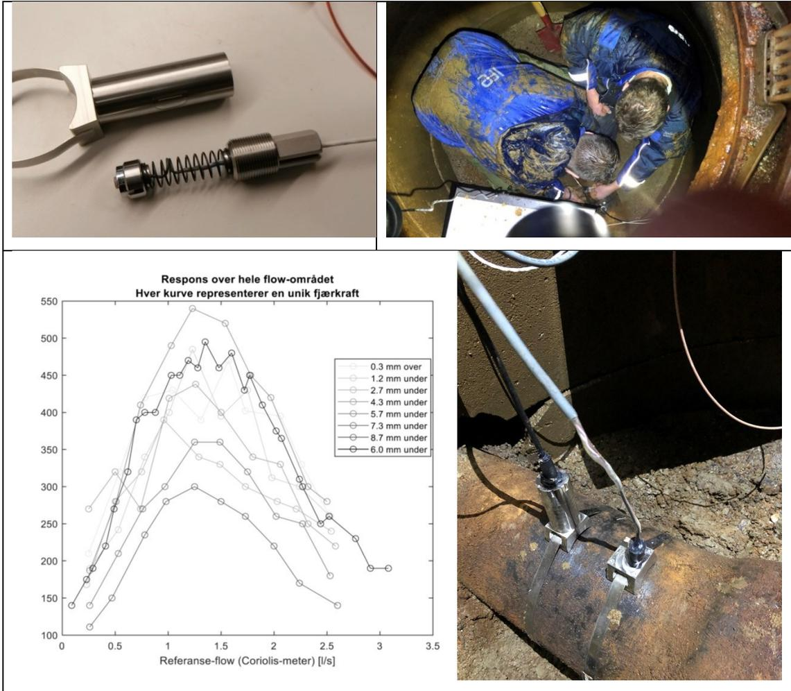
Figure 3-4 Installation of microphone & accelerometer from top position of the water pipe located inside of the manhole ~ 2 meters underground level - Response diagram of the sensors after installation (bottom left corner)
