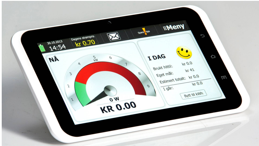
Figure 1.1: The eWave display being offered to Fredrikstad Energi's customers. The display is 7 inches across, and is based on the Android platform. Photo by Odin Media.
