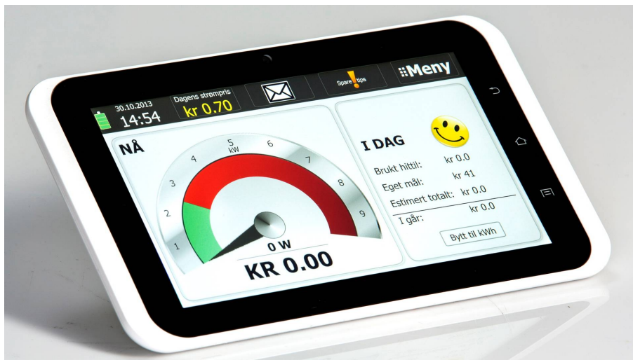
Figure 2.8: The eWave display being offered to Fredrikstad Energi’s customers. The display is 7 inches across, and is based on the Android platform. Photo by Odin Media.
