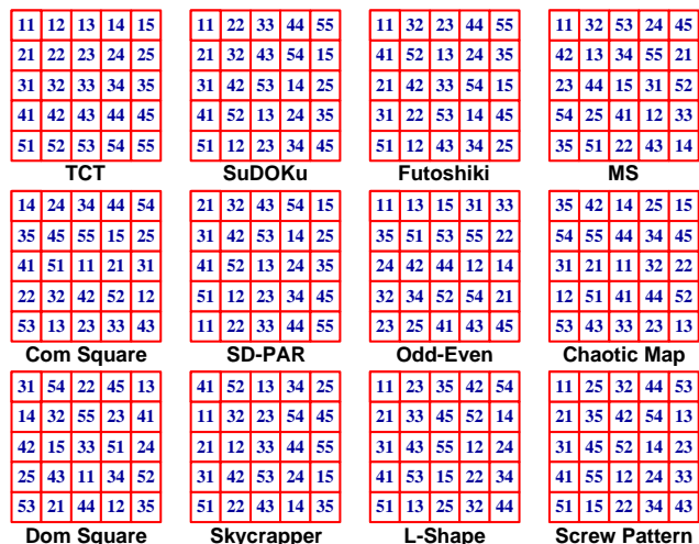
Figure 11. 5 × 5 PV Array Matrix Diagram of the various array configurations
