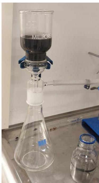
Figure 8 – Vacuum filter of Si@SiO<sub>2</sub>@GNS to drain out the water.
