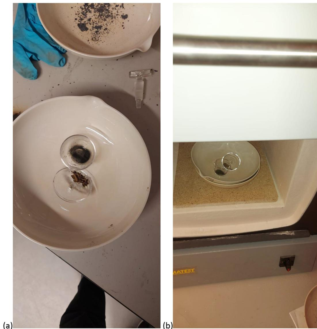
Figure 9 – (a) The burnt sample after calcination at 700°C (b) The sample obtained after calcination at 500°C.
