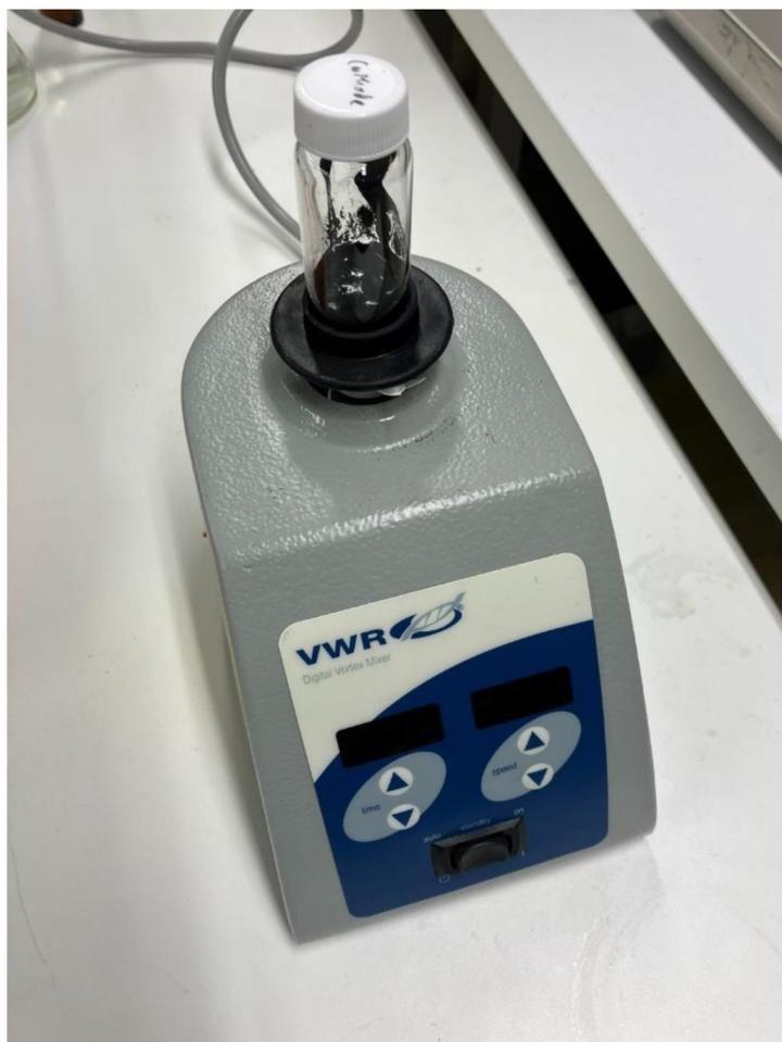
*Figure 11 – Homogenizer mixing the composition of electrodes to make slurry.*
