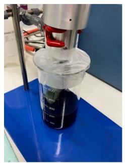
Fig 3. Ultrasonication of SiNPs and CNTs
