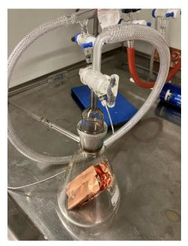
*Fig* 11. Setup to flush the glass flask with vacuum and argon.
