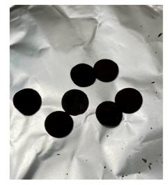
Fig 13. 10mm anodes punched from the fibre sheets.
