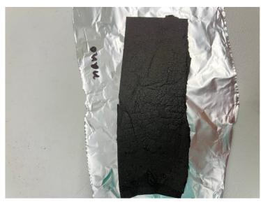
Fig 12. Carbonized composite fibre
