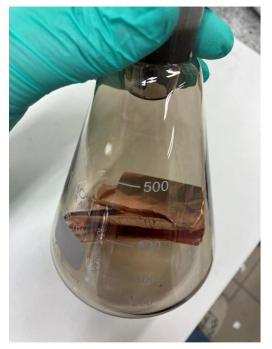
Fig 10. Glass flask with electrode material inside (wrapped in a film of copper)
