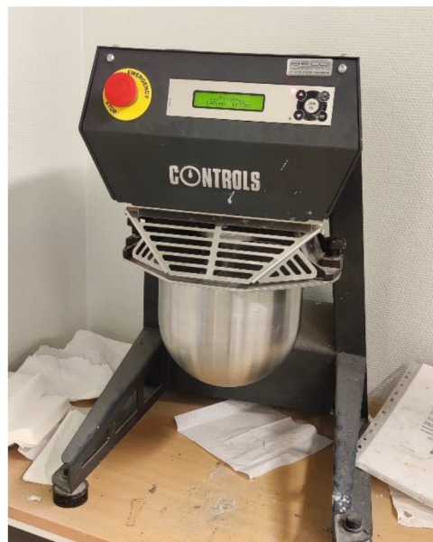
Figure 17. Cement benchtop mixer at Østfold University used to prepare shotcrete paste.
