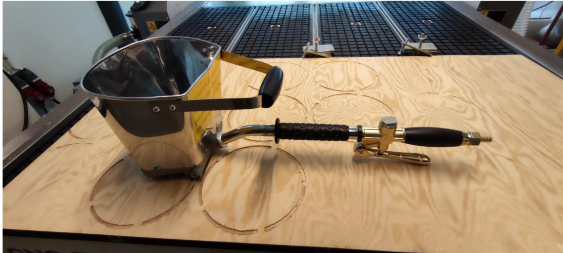
Figure 52. Lab scale shotcrete spray gun assembled at Østfold University College.
