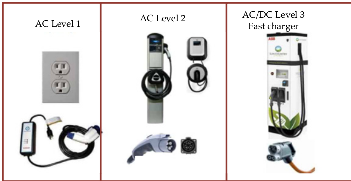
Figure 18. Voltage type level-based EV charging.
