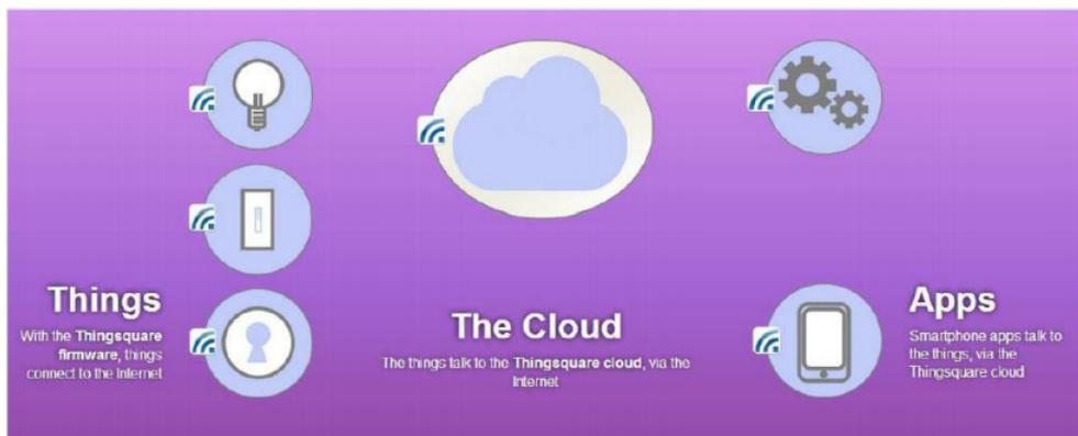
Figure 2.4: ThingSquare Architecture (Adapted from [5]).
