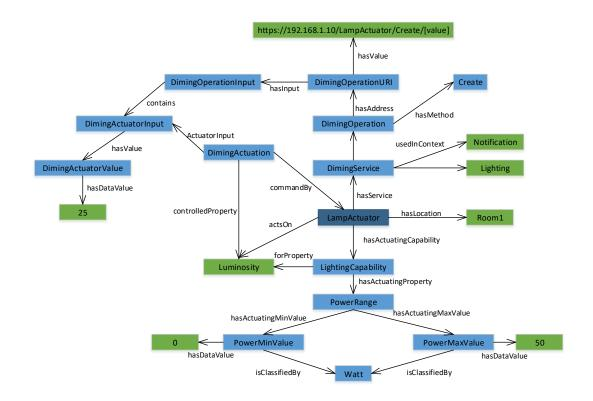
Figure 4.8: An Example Of Devices Ontology Instance
