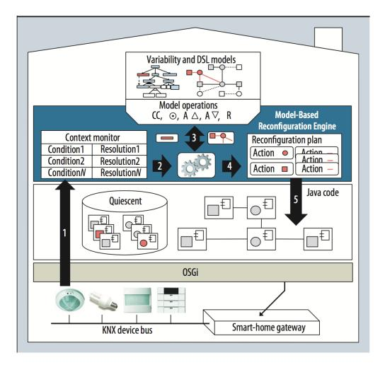
Figure 3.7: Model-based reconfiguration process. MoRE translates contextual changes into changes in the activation/deactivation of features. (Adapted from [27]).
