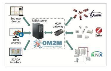
Figure 3.5: OM2M platform (Adapted from [10]).
