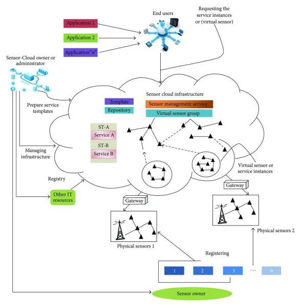
Figure 2.2: SensorCloud Architecture (Adapted from [9]).
