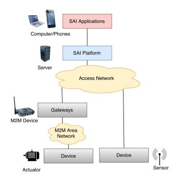
Figure 4.1: High level overview of the system architecture.
