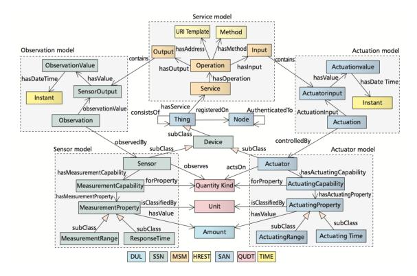
Figure 3.4: IoT-O ontology model (Adapted from [10]).
