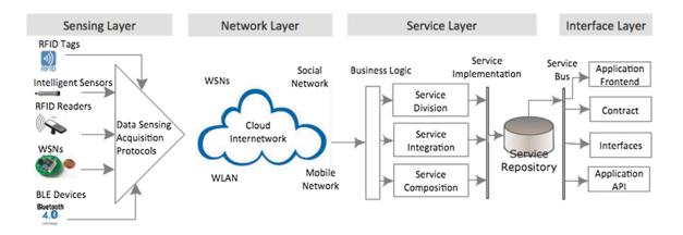
Figure 2.1: Service-oriented architecture for IoT (Adapted from [36]).
