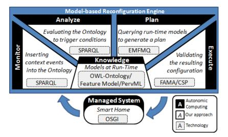
Figure 3.6: Overview of the runtime reconfiguration of Cetina et al. approach (Adapted from [27]).
