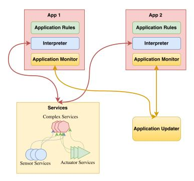
Figure 4.5: Overview of the communication between the applications and SAI platform.
