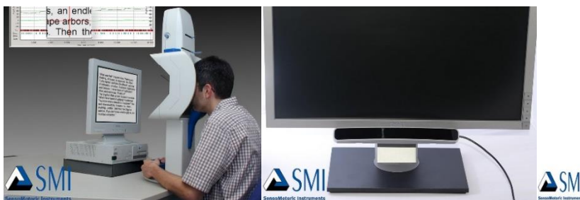
Figure 2.2 Images of three video-based eye-trackers produced by SMI (SensoMotoric Instruments). From left to right: Tower-mounted eye-tracker, remote eye-tracker attached to a monitor, head-mounted eye-tracker in the form of eye glasses.
