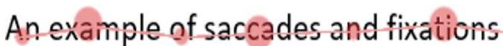
Figure 2.1 Example of tracked saccades and fixations while reading. The circles represent fixations and the lines represent saccades.
