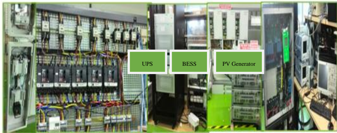
Figure 19. Experimental test set up with EMS controller and DES with load banks.
