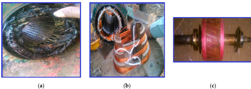
Figure 6. (a) Old scrap motor. (b) Redesigned winding arrangement for the proposed multifunctional motor. (c) Squirrel cage rotor (rotor of the old machine).
