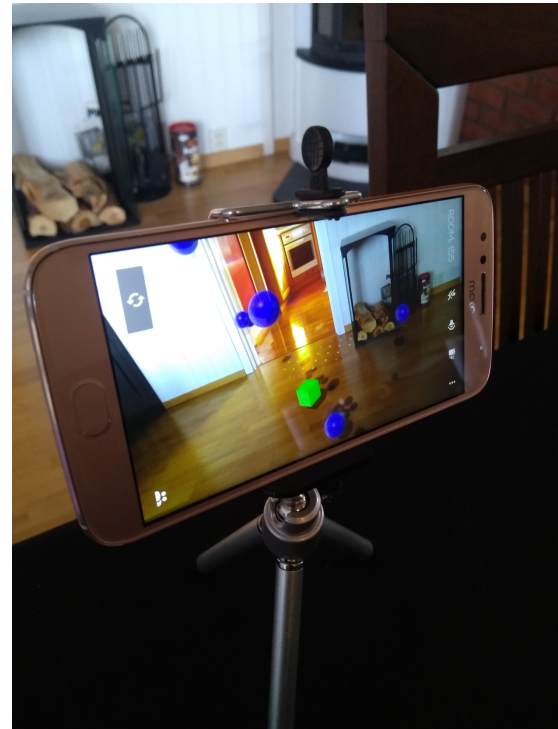
Figure 4.23: Screenshot of prototype during a shared augmented reality session. The green cube being visible indicates that the prototype is in debug mode.
