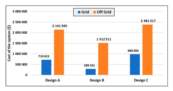
Figure 10. Comparison of grid/off-grid connection for optimal designs.
