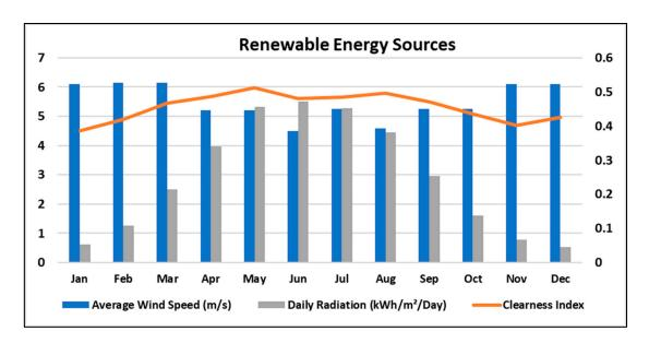
Figure 4. The average monthly renewable energy source (RES) generation data at DTU-Risø.
