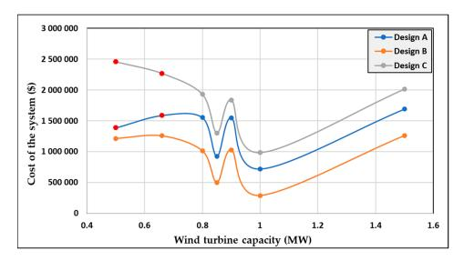
Figure 8. Comparison of grid connected system for design A, B, and C.
