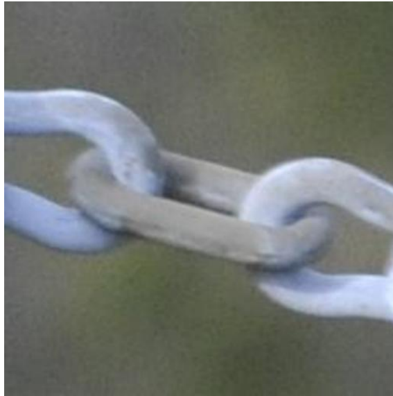
Figure 3.5: Image of normal chain shackles which CSRN predicts 80% worn
