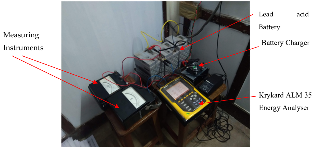
Figure 8. Experiment setup for finding battery charging efficiency.
