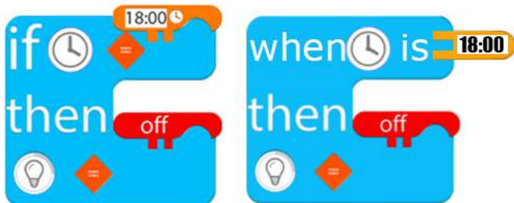
Figure 6.9: Left: A common timer structure from the second iteration prototype. A timer relationship always requires a clock -, equals -, and a timer block. Right: Mock up of new timer block. Here the clock and operator is fixed, the user only selects the time. If not for spacing, it could also be more fixed and read "when the time is...".
