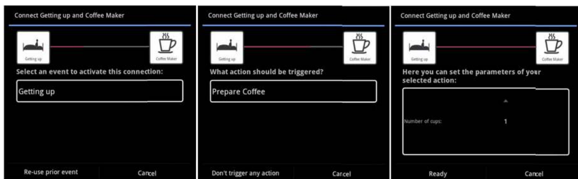
Figure 2.4: The homeBLOX wizard. A two step creation of a relationship between devices.
