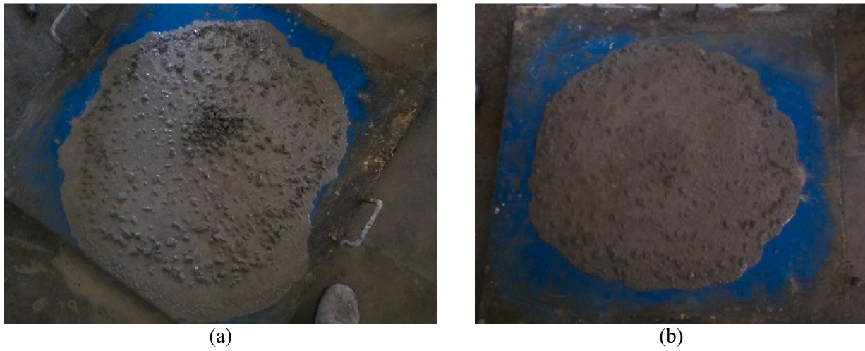
Fig. 29. Using different designs to observe the effect of instability in concreting in the specimens with (a) unstable concrete, and (b) stable concrete.
