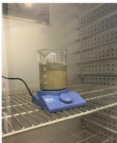
*Fig 6. The SiNP-CNT-GO suspension in the oven on a magnetic stirrer.*
