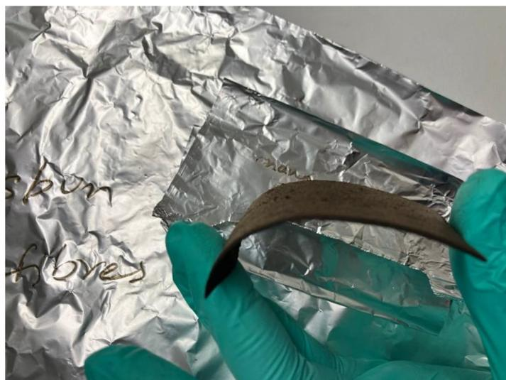
*Fig 8. Stabilized composite fibre*
