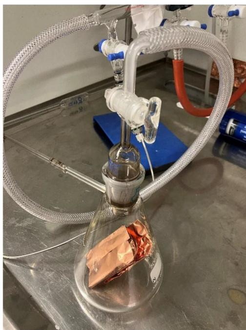
*Fig 11. Setup to flush the glass flask with vacuum and argon.*
