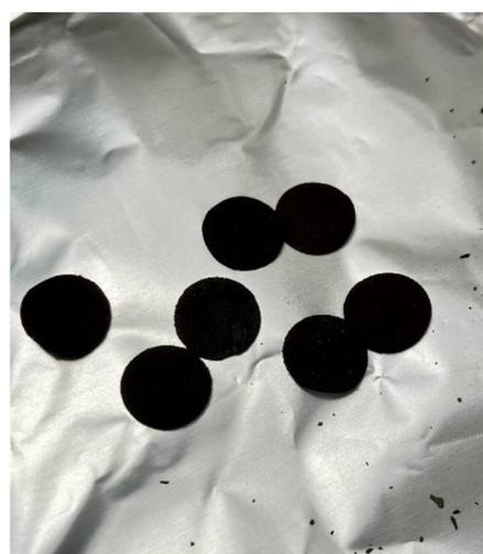
Fig 13. 10mm anodes punched from the fibre sheets.
