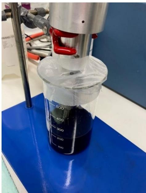
*Fig 3. Ultrasonication of SiNPs and CNTs*
