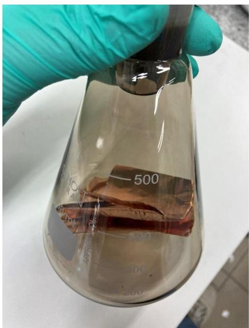
*Fig 10. Glass flask with electrode material inside (wrapped in a film of copper)*
